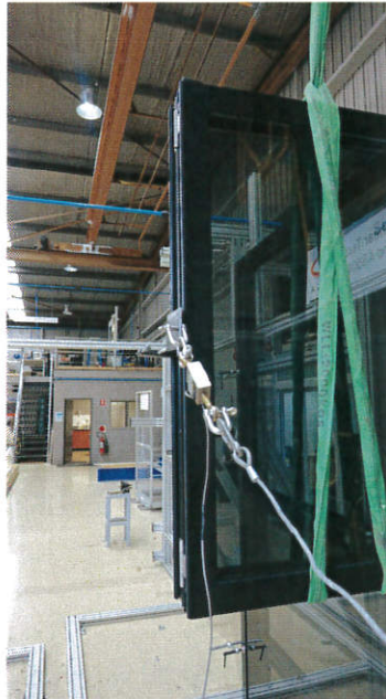
Figure 4: Set-up of point of pull (strap is loose)
